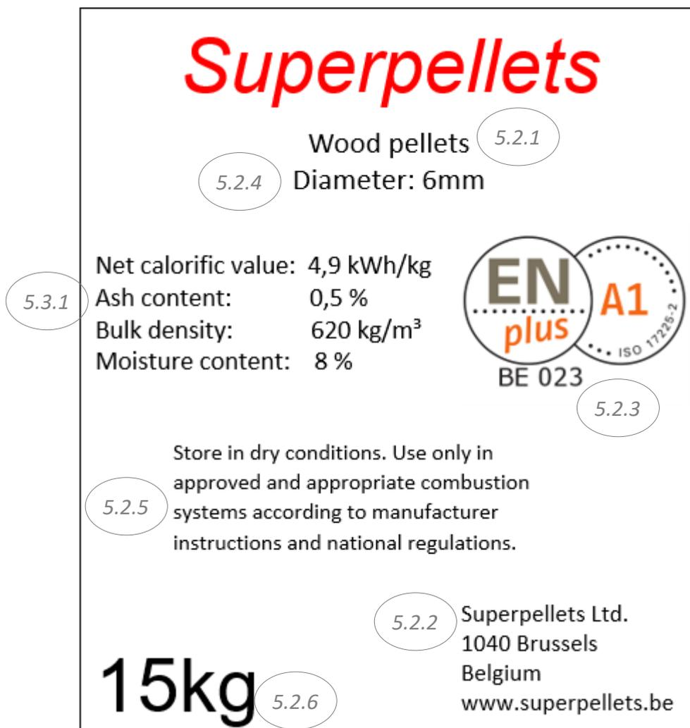
**Figure 1:** Illustration of a bag design
